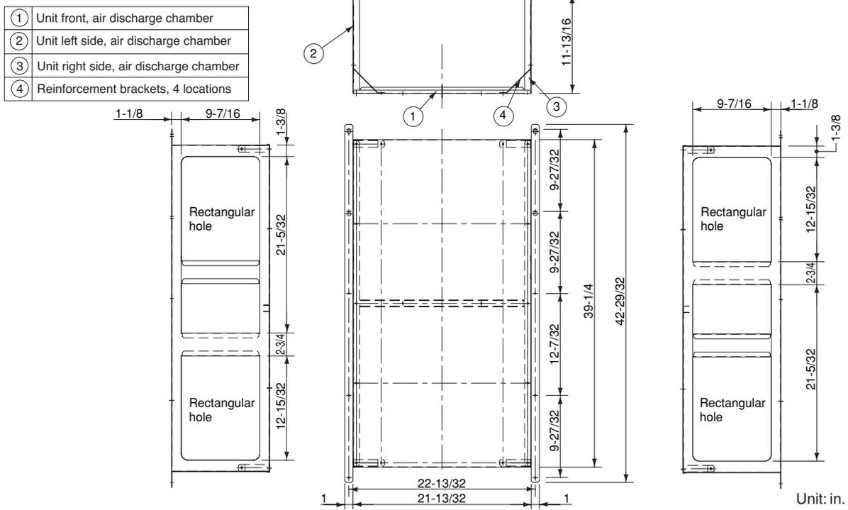
**2-6. Dimensions of Outdoor Unit with Air-Discharge Chamber (field supply)**
