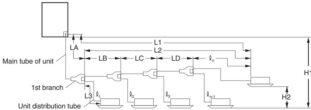
Note: Do not use commercially available T-joints for the liquid tubing.
