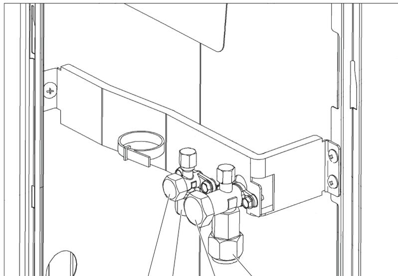
Tightening torque for valve stem cap: 160 – 180 lbs · in. ④      ① Tightening torque: 590 – 710 lbs · in.
