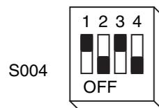
“5” is set as the central control address for indoor unit group 0, and “7” is set as the central control address for indoor unit group 2.
